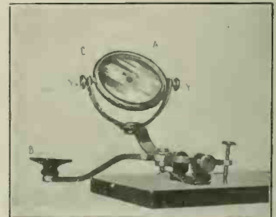
A Simply Made "Heliograph" Similar to That Used by Army Signal Corps. It Will Prove Very Effective for "Boy Scout" Signaling Work.
