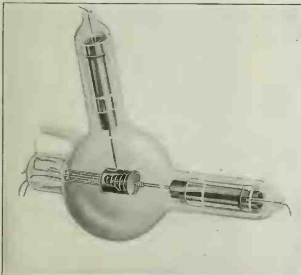
Fig. 2. Vacuum Tube Oscillator for Generating or Amplifying Radio Currents—The "Dynatron."
